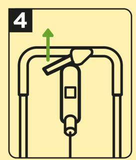
Start to walk and pull the handle upwards to begin spreading.
